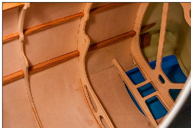
In the cockpit area the fuselage is planked with 0,4 plywood so there is no glassfiber laminate visible.
