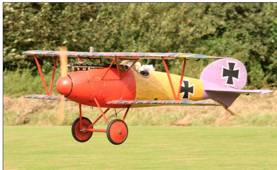
With our albatross, one can take off with quarter throttle, and with even less throttle continue flying. This way the ZG 80 has a very realistic sound. The six cylinder Mercedes engine at maximum take off power was only making 1500 RPM.
