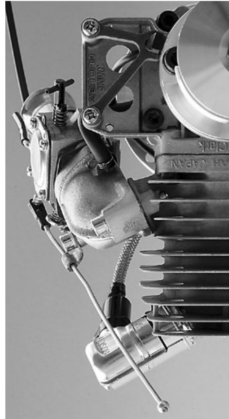
The pictures show the cast aluminium intake bend #4587 and the intake trumpet with flange #0081.
