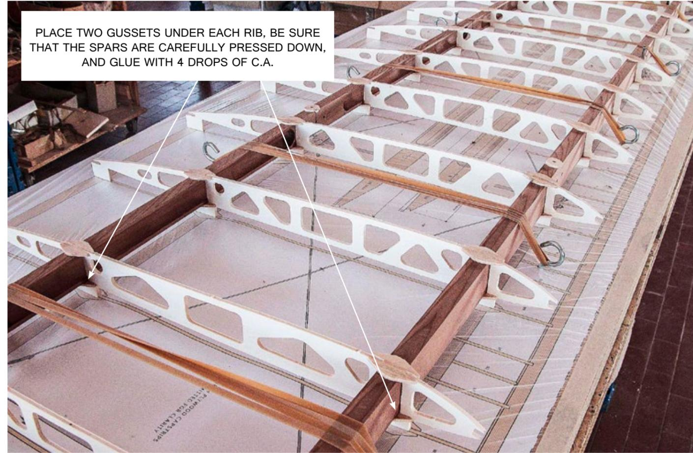
PLACE TWO GUSSETS UNDER EACH RIB, BE SURE THAT THE SPARS ARE CAREFULLY PRESSED DOWN, AND GLUE WITH 4 DROPS OF C.A.
