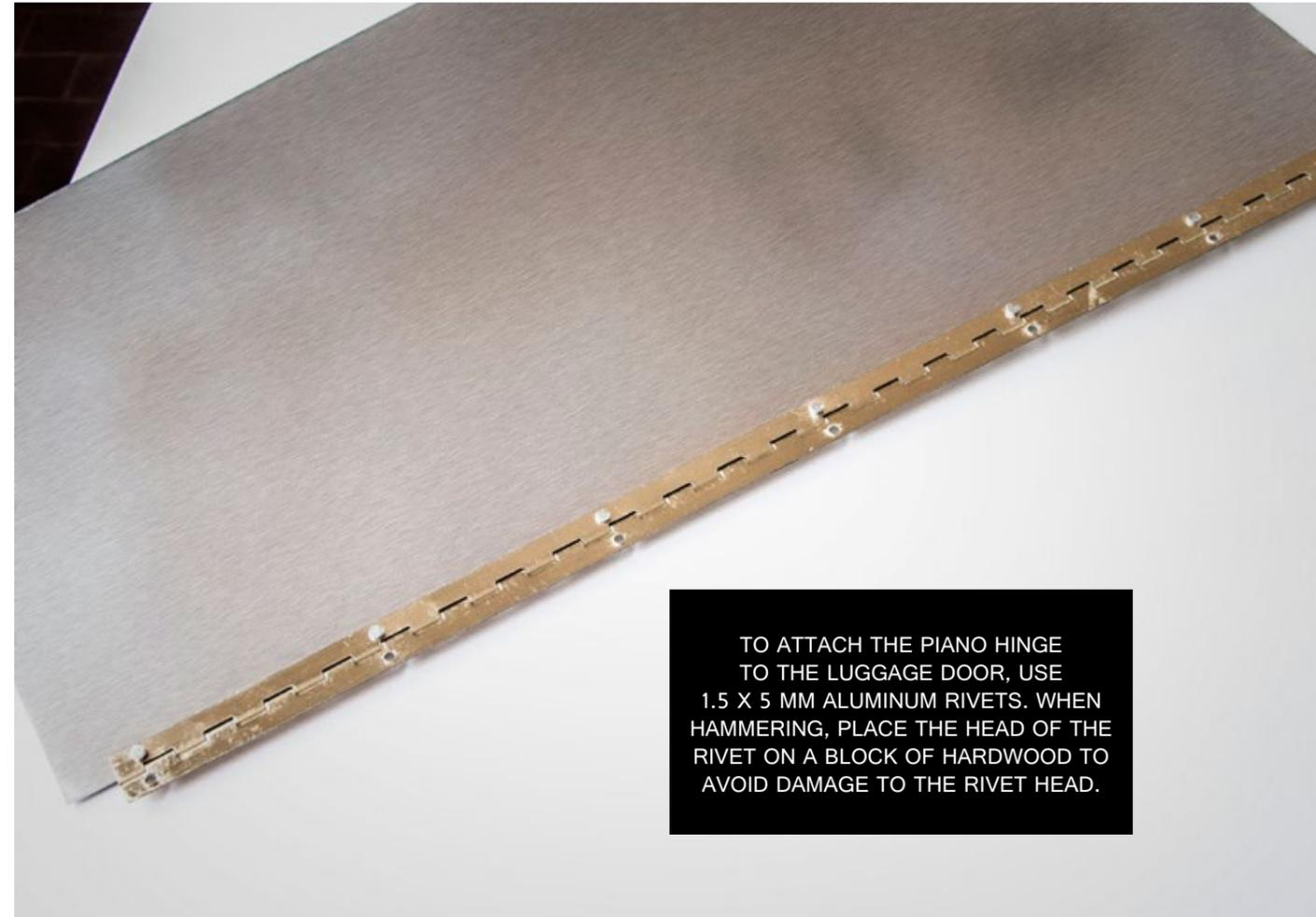
TO ATTACH THE PIANO HINGE TO THE LUGGAGE DOOR, USE 1.5 X 5 MM ALUMINUM RIVETS. WHEN HAMMERING, PLACE THE HEAD OF THE RIVET ON A BLOCK OF HARDWOOD TO AVOID DAMAGE TO THE RIVET HEAD.
