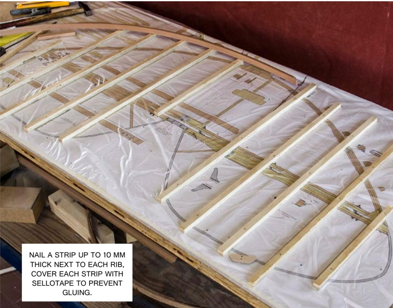
NAIL A STRIP UP TO 10 MM THICK NEXT TO EACH RIB, COVER EACH STRIP WITH SELLOTAPE TO PREVENT GLUING.
