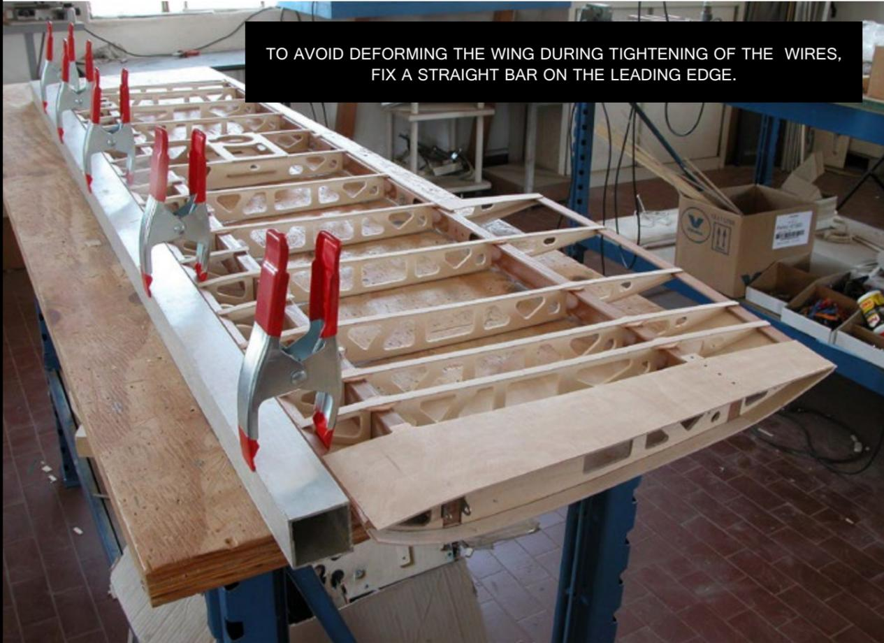
TO AVOID DEFORMING THE WING DURING TIGHTENING OF THE WIRES, FIX A STRAIGHT BAR ON THE LEADING EDGE.
