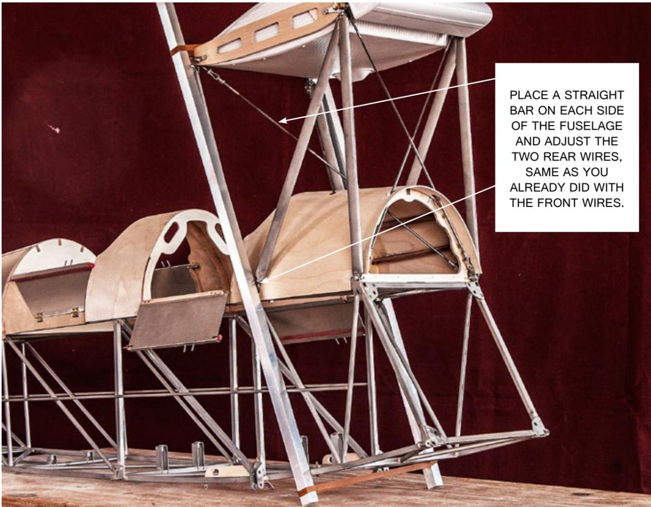
PLACE A STRAIGHT BAR ON EACH SIDE OF THE FUSELAGE AND ADJUST THE TWO REAR WIRES, SAME AS YOU ALREADY DID WITH THE FRONT WIRES.
