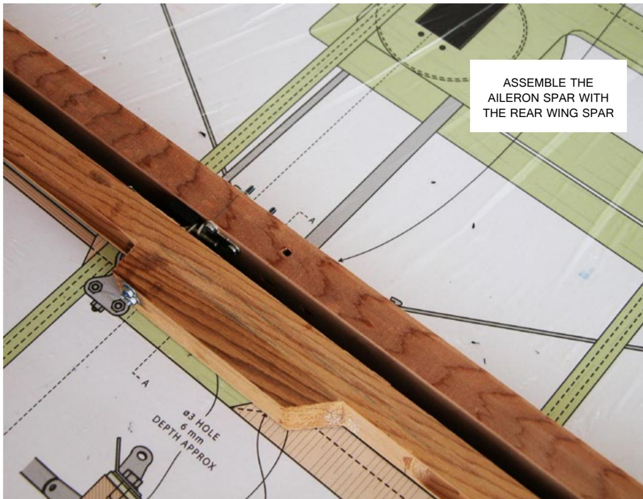
ASSEMBLE THE AILERON SPAR WITH THE REAR WING SPAR
