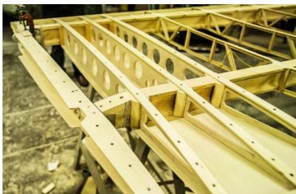
Bottom wing of a real Tiger Moth under restoration, the upper plywood sheeting is modified now to represent the original.
