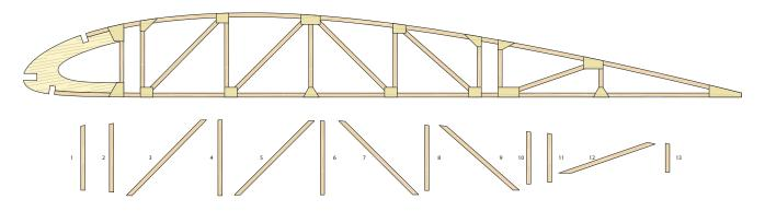
Cut a set of bracing strips using the nylon mold as reference.
