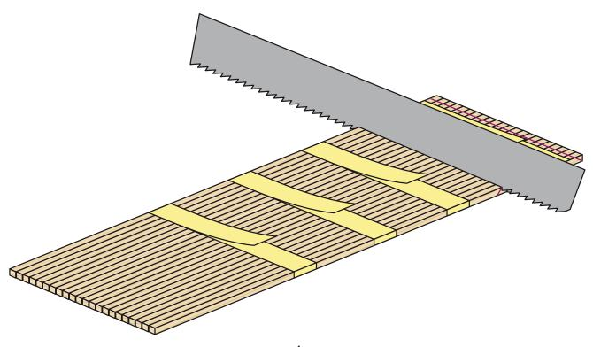
4. Saw a complete set of bracing strips. You can use also a disk saw with angle regulation.
