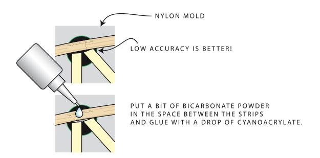
Note: the ribs shown are of the Bücker kit. For the Piper ribs use the same procedure.
