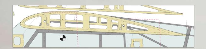
For the first flight, place the CG to 140 mm from leading edge and insert the adjusting pin as in the image. In any case the Grasshopper can fly in a wide range of trim, in order the flight performance you prefer.
