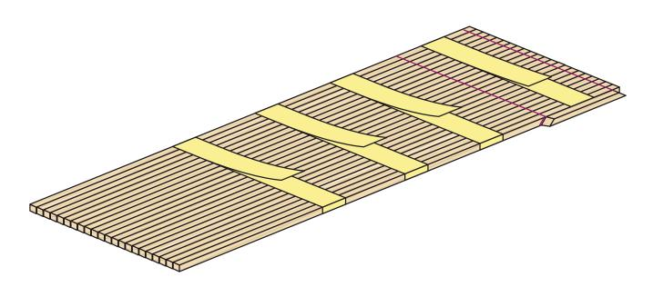
3. Allign a bracing strip to side and trace the referring lines.
