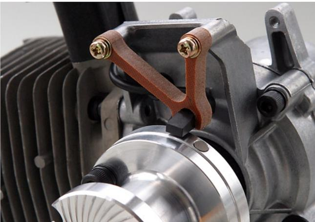
This is how the pickup should be.
