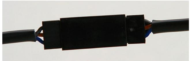
Take care with plugging together the JR-plugs and sockets by noting that the colours should line up on opposite sides. It is possible with a little extra effort to push these together with reverse polarity. No damage will be done but the ignition will of course be dead. I tape these plugs and sockets with insulation tape for additional safety.
