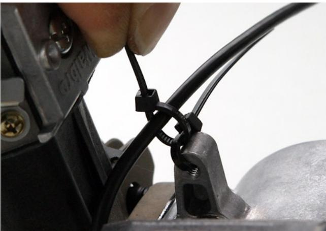
... and with the second tie the cable is fixed to the first.
