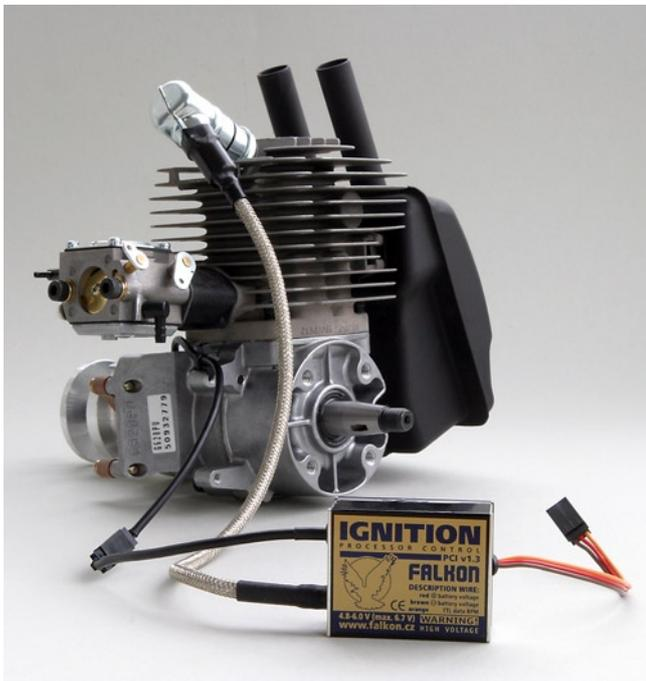
Please fit the cables very carefully into your model, especially the high tension cable, as this will not contain the 21,000 volts if it is damaged due to scuffing against the cowl inner surface. If the screening flex is damaged due to scuffing when threaded through a GRP cowl opening, it will not be long before the inner insulation is damaged also. Then the HT will short out to the screening flex and this may cause massive radio interference and will of course lead to an ignition cutout.
