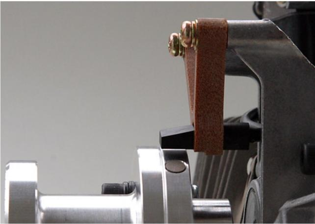
Looked at from the side, the pickup position is even less critical, you see here the middle position. Although 2 mm forwards or backwards will work perfectly well.
