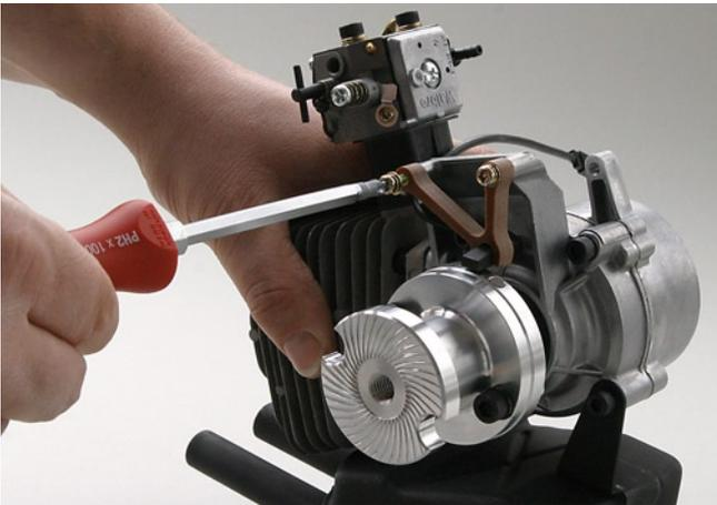
Now fit the pickup head with the power coil screws as shown. The ignition timing is automatically correct and cannot (and need not) be adjusted.
