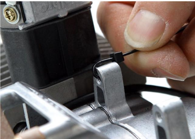
Use the nylon cable ties to secure the pickup cable. The first cable tie is shown here ...
